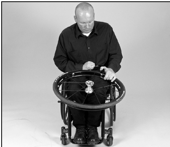
Image 17: Pull the tire edge over the rim
