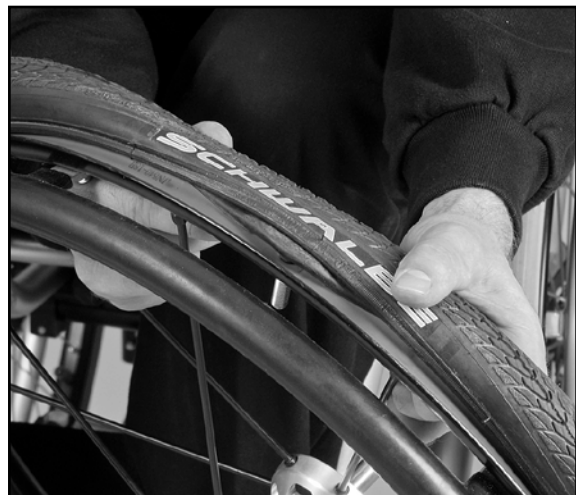
Image 18: Pull out the tube
