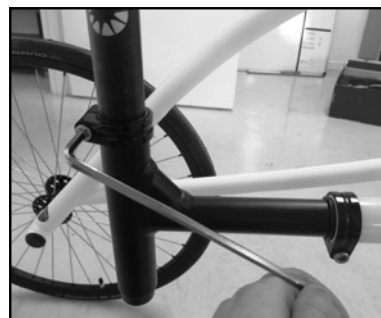
Image 7 Loosen the bolt to height adjust
