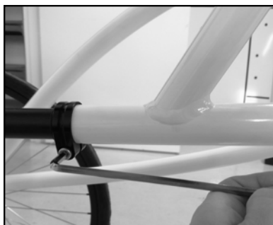
Image 5 Loosen the bolt to depth adjust
