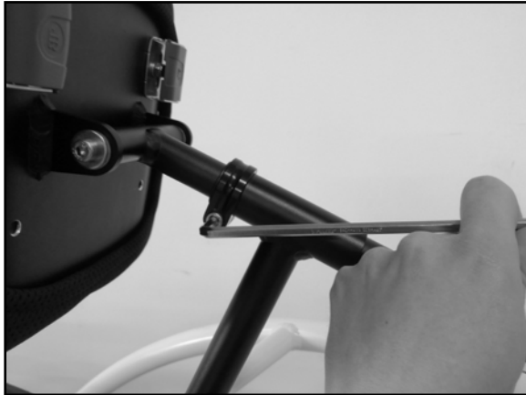
Image 11 Loosen the bolt to adjust chestplate
