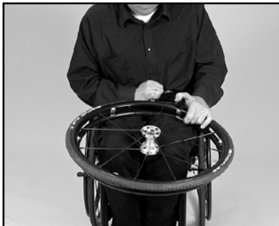
Image 18 Pull the tyre edge over the rim
