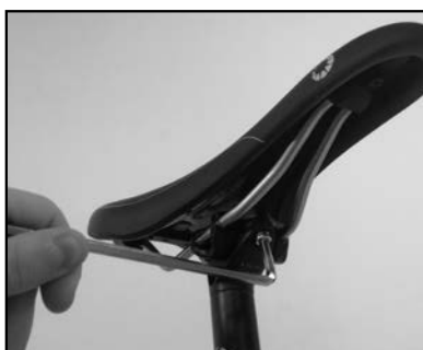
Image 8 Loosen the bolt to angle adjust
