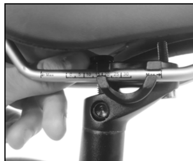
Image 9 Turn the bolt to angle adjust
